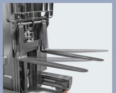
Forks can tilt forward/backward for easy loading
