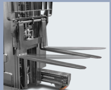
Forks can tilt forward/backward for easy loading
