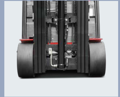
Front dual separated motors
