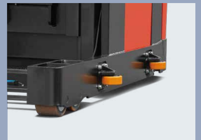
Rail guidance rollers (Opt.) can be fitted to the truck for VNA working
